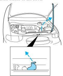
3. Lift the hood and secure it with the prop rod.
